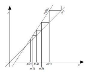
Figure 3.4: Iterating f(x) = ax + b with a > 1.
