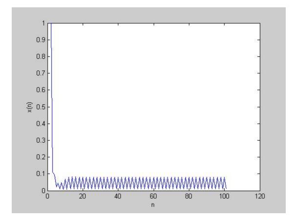
Figure 4.1:  $x_{n+1} = .1x_n + \frac{.001x_n + x_{n-1}}{300x_n + 3x_{n-1}}$  has prime periodic two solutions
